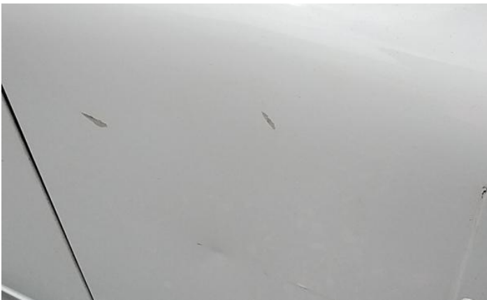
5: Wing nsf Scratched Over 25mm Thru Paint
